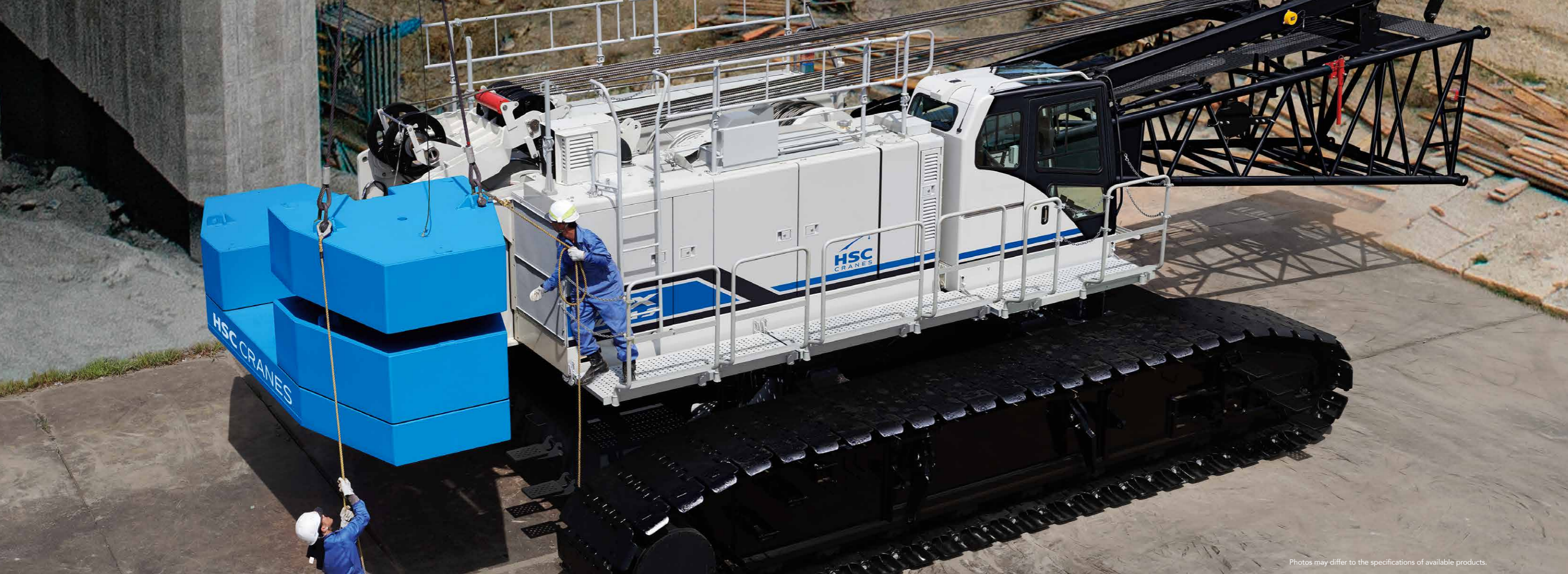
Counter weights and boom can be transported together
