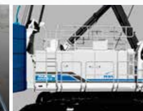
Catwalk with handrails and folding type upper house handrails
