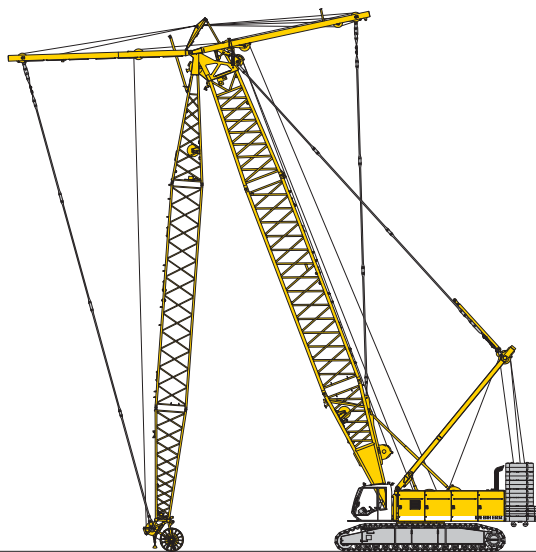
Erecting of main boom and luffing jib
