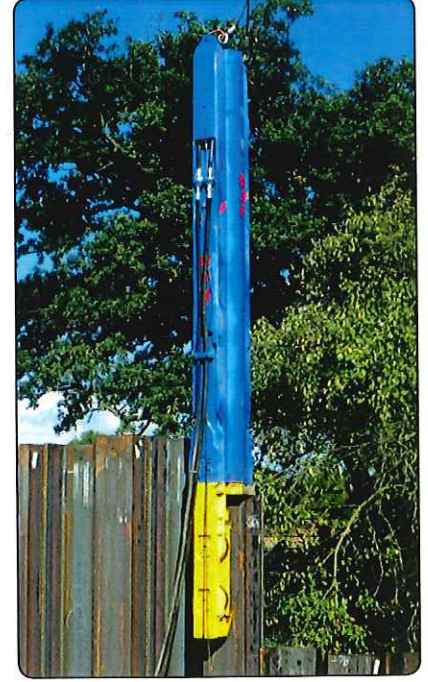
Above: Various SL30 Hammers fitted with legs and inserts for diving sheet piles. All are shown in crane suspended operation and powered by BSP Power Packs.
